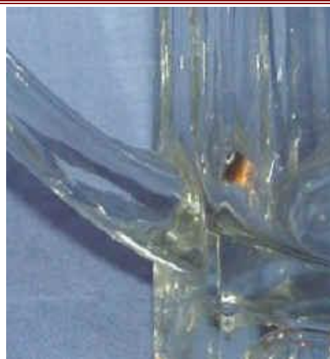
Left, pressed glass handle showing mold marks at the centerline of the handle, continuing on the body. Right, typical handle attachment on a pressed glass stein, handle and body are a single piece of glass.
