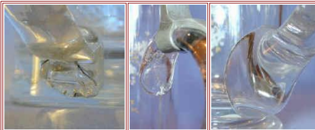
Three examples of attached handles on blown glass steins. Earlier examples (left) are much less regular than those achieved toward the latter part of the 19th century (middle and right).
