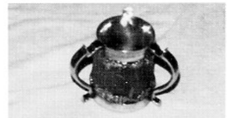
Figure 17. Buffing now restores the highlights, while leaving carbon in cracks and crevices.
