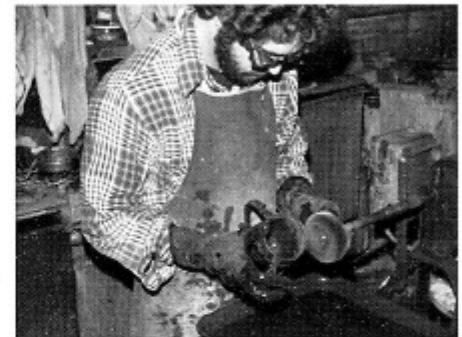
Figure 15. A dip-solution and scratch-brushing removes rust from the cup.
