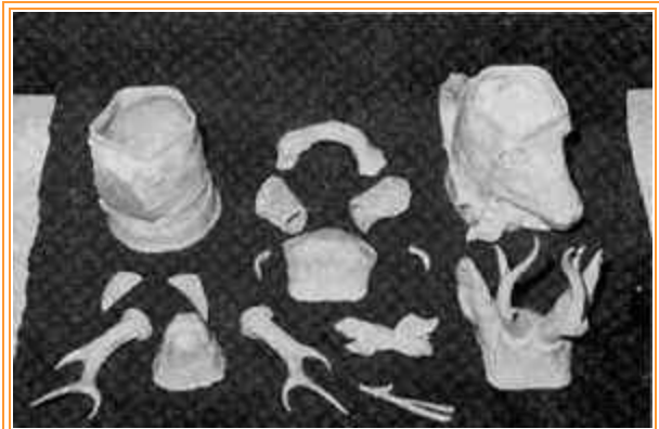
Fourteen separate pieces that make up the stag stein (left); Assembled and lead-glaze fired on right.
